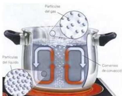
Something similar happens when we heat water in a casserole. The flame or electric plate heats the inferior part of the casserole and it causes a dilatation of the hot water in the bottom, which becomes less dense than the rest of the water. As a consequence, the hot water goes up and the cold water occupies the lowest space.
