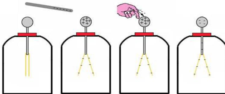
The electroscope keeps being neutral, but the closest area to the positive rod has an excess of electrons and the area which is further has a lack of electrons. The closest area to the negative rod has a lack of electrons and the furthest area has an excess. You can charge the electroscope as it is shown in the pictures.
