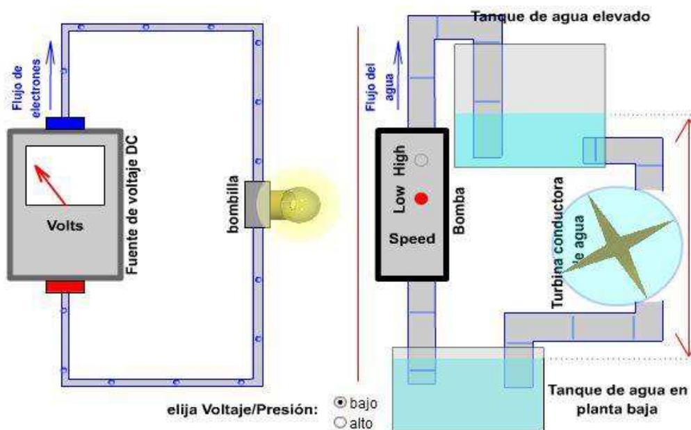
Now, look at the electric circuit. It is easy to identify the equivalent to the flow: the intensity of the current. Just as like water, that needs a pump that impulses it to continue its flow, charges need a booster that allows it to continue flowing. This device is called a generator.
