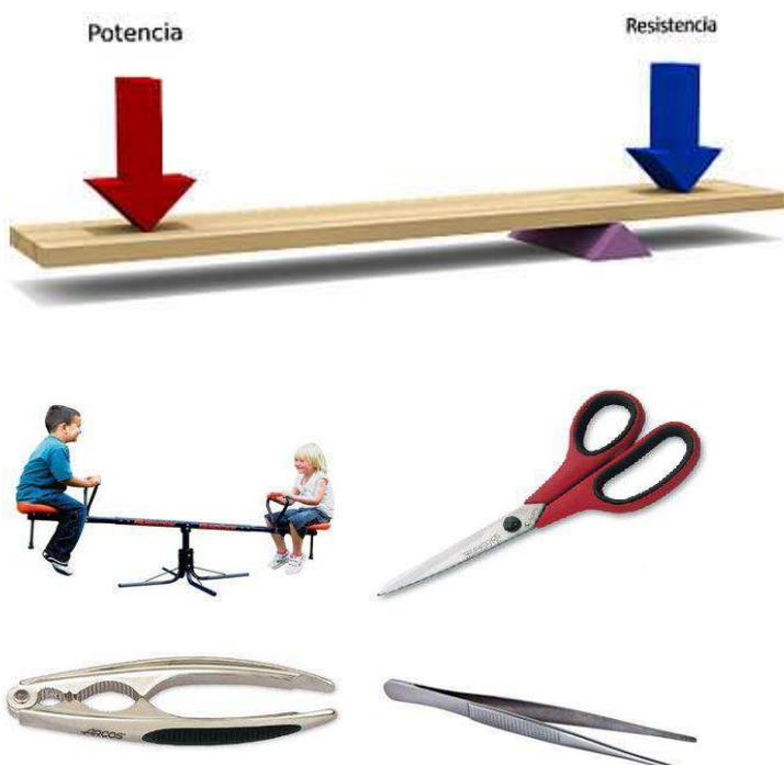
Some levers allow us to reduce the force we need to apply to do a task, as in the case of the nutcracker. This instrument is used to break the shell of a nut, something that would be more difficult if we tried to do it only with our hands. The scissors and the pin are similar examples.
